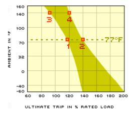
Performance characteristics are based on room temperature (77°F). Consult derating curve at left for ambient temperatures significantly higher or lower than standard room temperature.
