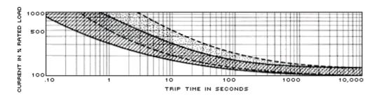
Dotted Lines: Small Frame P series PDA, PDM (10 amps and below) Solid Lines: Small Frame P series PDA, PDM (above 10 amps)
