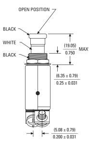
Note: 2TC27 amp rating marking is rotated 180 degrees from illustration \*\*\* 2TC27 dimension is 1.125" (28.57mm) Max
